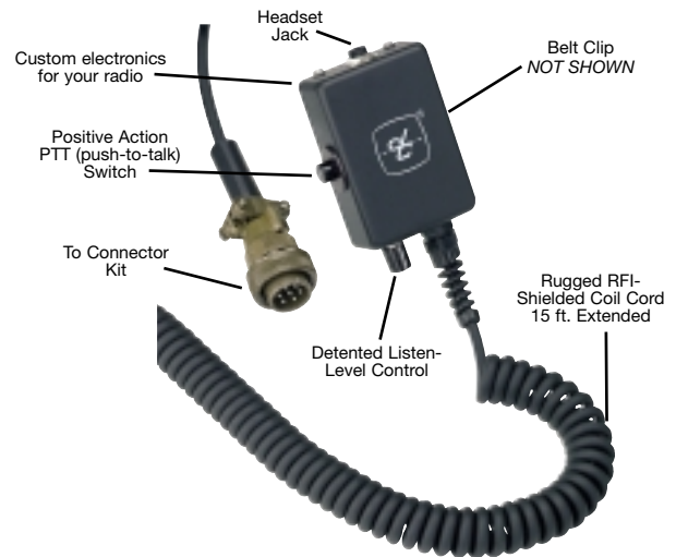
Attaches to accessory port. Retains hand microphone.
